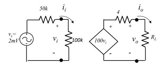
1. For the following circuit, determine the value of  $R_L$  to maximize the power gain for this circuit. Provide a proof. Which value of  ${\cal R}_{\cal L}$  makes the better design and why?
